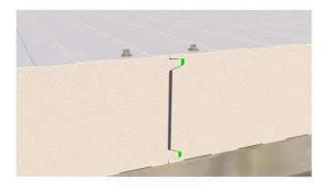
In Proceed in similar fashion with the installation of the subsequent panels to the end of the wall.
