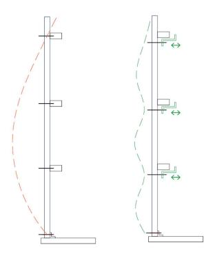
If the panel were fastened at the ends only, a curvature due to thermal expansions, such as the one shown in red in the figure, would occur. Normally, fastening systems provided for the panels lead to a curvature similar to that shown in green.
