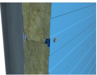
Similarly, proceed with the installation of the subsequent panels to the top of the wall.
