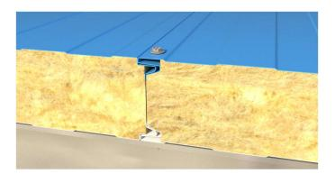
Proceed in similar fashion with the installation of the subsequent panels to the end of the wall.
