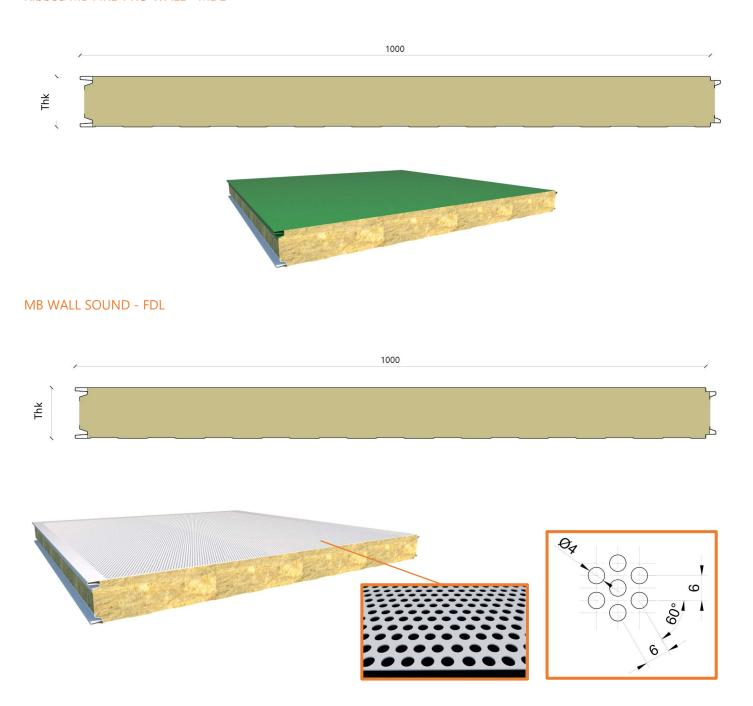
To increase the acoustic properties, the metal support on the inner side of panels is perforated with 4 mm diameter holes (R4T6), arranged in a triangle with centre distances of 6 mm, to generate an intermittent arrangement.
