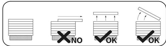
If necessary, depending on the size and weight of the individual panel, it is advisable to provide suitable mechanical lifting devices, such as **suction cup lifters** or special **grippers/jaw clamps**.
