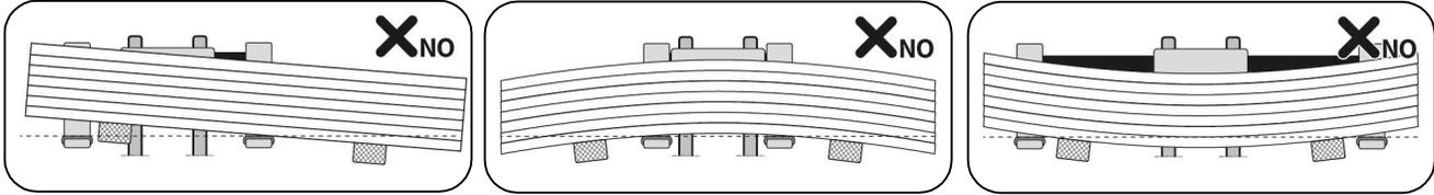
Handling of panels on site must be carried out with suitable **lifting systems** that have been **adequately designed and dimensioned** so as not to cause damage to the material during assembly.
