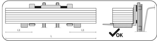
If the parcel is lifted in an unbalanced manner, not taking into account the correct gripping points, there is a risk of consequences such as the parcel falling or the panels being deformed and damaged.
