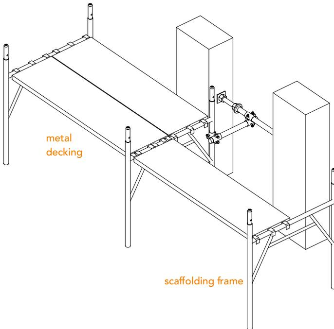
In special cases, when other types of anchorages are not permitted, force screws can be used, provided their working is checked and monitored while in use.
